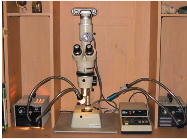
Figure 4. Housed in a sturdy protective cabinet, the author's gemological photomicrographic system uses a trinocular arrangement so that the camera remains in place when the system is being used as a binocular microscope. Note that this custom-made darkfield and transmitted light system uses two fiber-optic illuminators (with a white film canister diffuser on the wand that is lit), but it is also easily set up for applications with polarized light, shadowing, and ultraviolet illumination. Photo by Maha Tannous.
