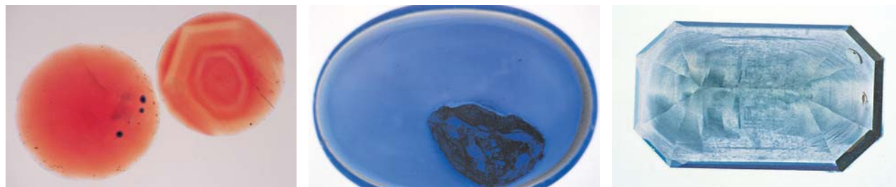
Figure 26. These three photos were all taken in an evaporating dish using partial immersion with methylene iodide and diffused transmitted light. On the left, one of the 4.2 mm bulk-diffused Madagascar sapphires shows the yellow rim indicative of beryllium treatment, whereas the other reveals alteration of the originally pink hexagonal zoning to orange and yellow. The center image details irregular spotty coloration on the surface of a 7.1-mm-long bulk-diffused blue sapphire cabochon. And the image on the right shows structurally aligned, internally diffused blue “ink spots” in an 8.6-mm-long heat-treated sapphire from Rock Creek, Montana.
