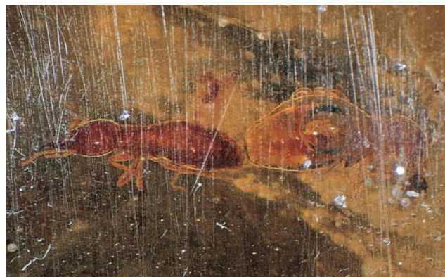
Figure 27. Holding a soldier and a worker termite captive, this copal from Madagascar is badly scratched, which drastically affects the quality of the image (left). However, spreading a droplet of sesame oil (R.I. 1.47) over the surface creates a “quick polish” on the copal, so the termites can be photographed clearly (right). Magnified 5×.
