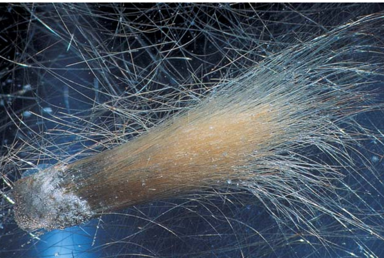
Figure 13. This image showing a comet-like sprig of rutile in quartz was created by light painting using a pinpoint fiber-optic illuminator. Magnified 10 \times .
