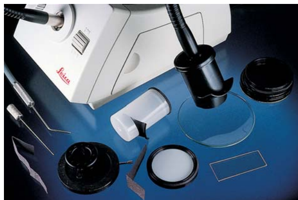
Figure 6. This collection of lighting accessories would be found in any complete gemological photomicrographic laboratory. Shown here are a single-wand fiber-optic illuminator; a pinpoint fiber-optic illuminator with two end attachments; two Polaroid plates and a first-order red compensator; a white diffusing plate; two iris diaphragms for shadowing; two modified film cans and two black paper strips for hot spot control; and a shallow glass evaporating dish for partial immersion if needed. Photo by Maha Tannous.
