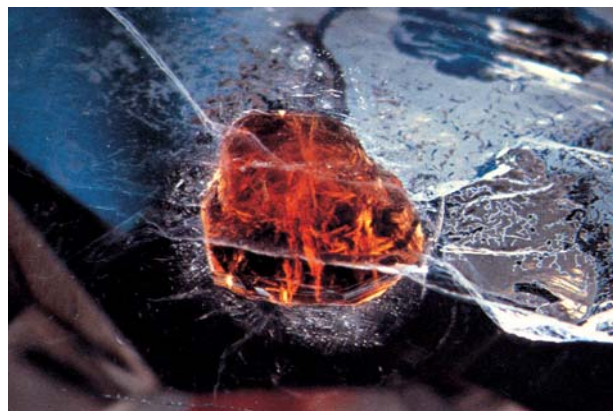
Figure 15. Darkfield lighting is used to study transparent-to-translucent included crystals, small fluid inclusions, and partially healed cracks, all of which are illustrated in this image of a spessartine garnet in quartz. Magnified 3 \times .
